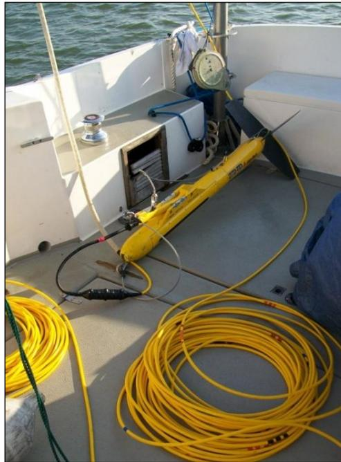
Figure 8. Sonar Edgetch 272TD
