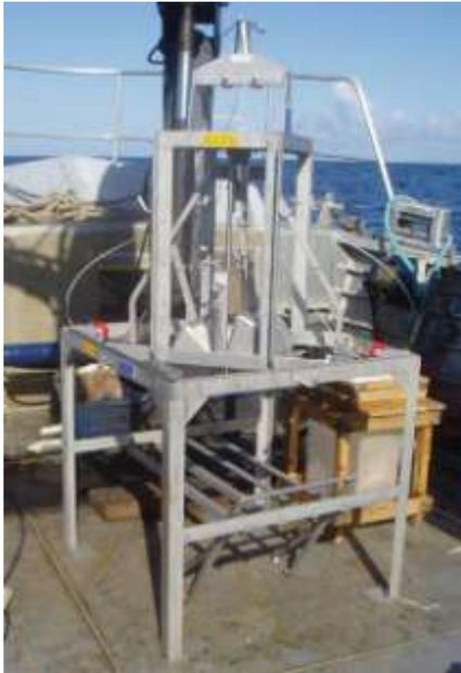
*Figure 8: Benne Smith Mc-Intyre (Cliché TBM)*
