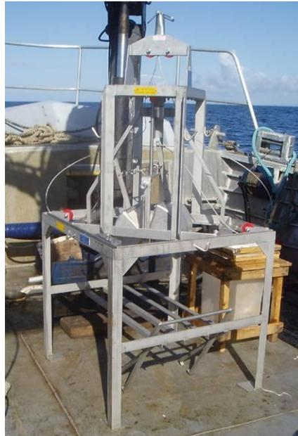
*Figure 8: Benne Smith Mc-Intyre (Cliché TBM)*
