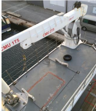
5 + 1.5 t SWL deck crane
