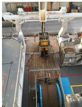
Working deck with ROV ready
