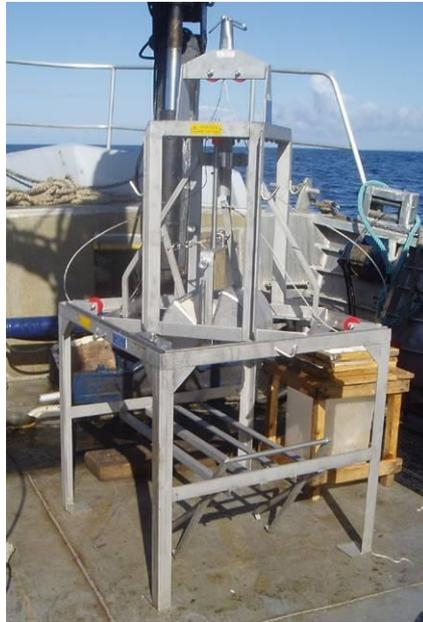
*Figure 8: Benne Smith Mc-Intyre (Cliché TBM)*
