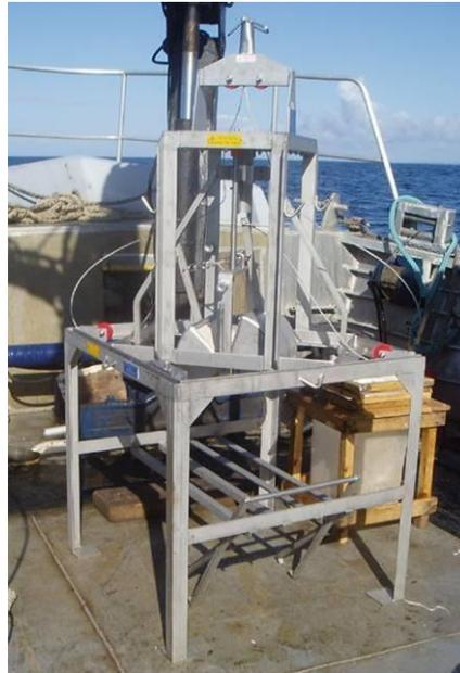
*Figure 8: Benne Smith Mc-Intyre (Cliché TBM)*
